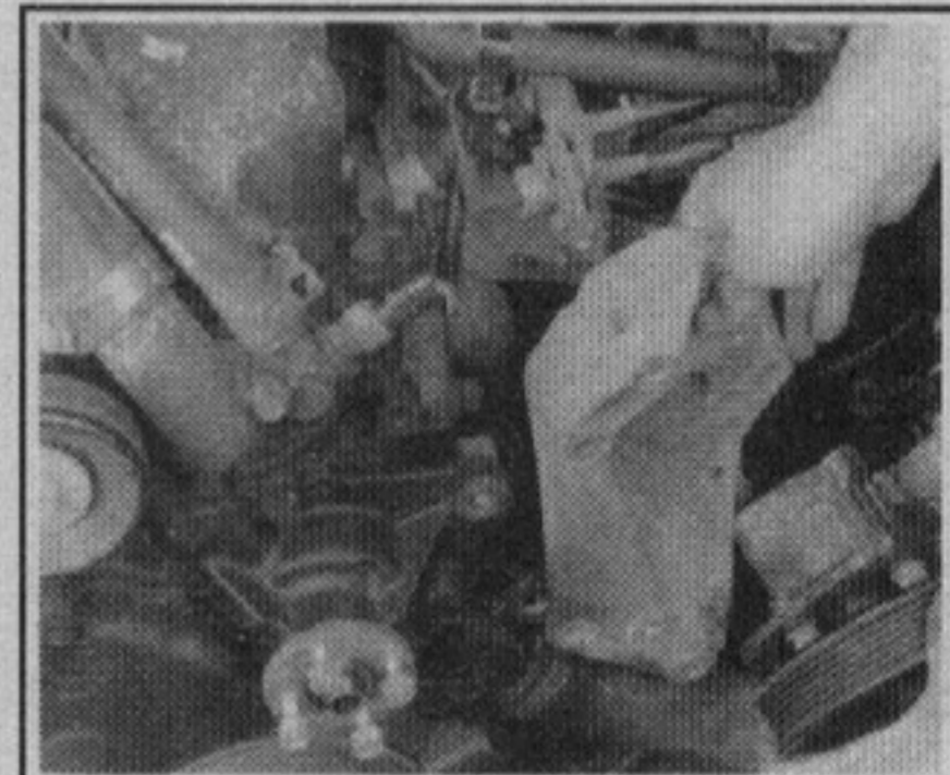
Fig. 92 Remove the power steering pump mounting bracket
