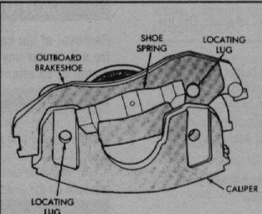
Fig. 31 Tilt the caliper outboard to remove
