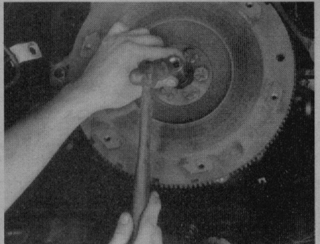
Fig. 13 Tap gently to install the pilot bearing
