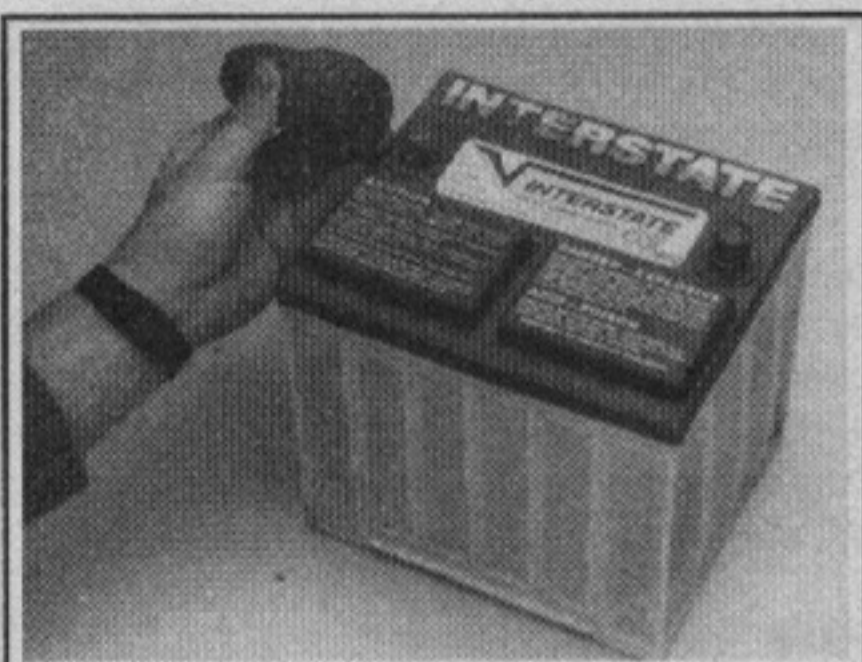
Fig. 44 The underside of this special battery tool has a wire brush to clean post terminals
