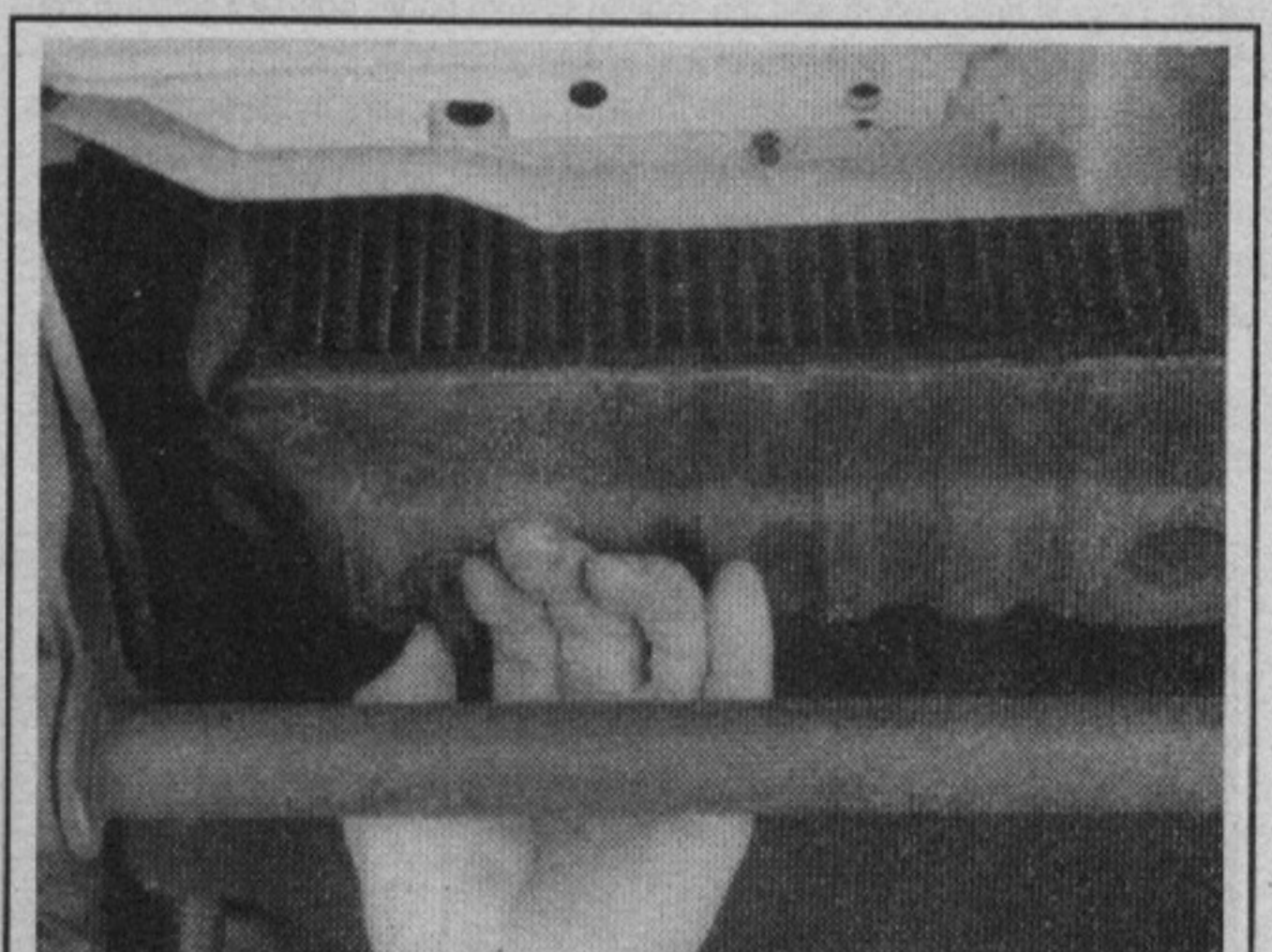
Fig. 119 Drain the radiator by loosening the petcock at the bottom of the radiator
