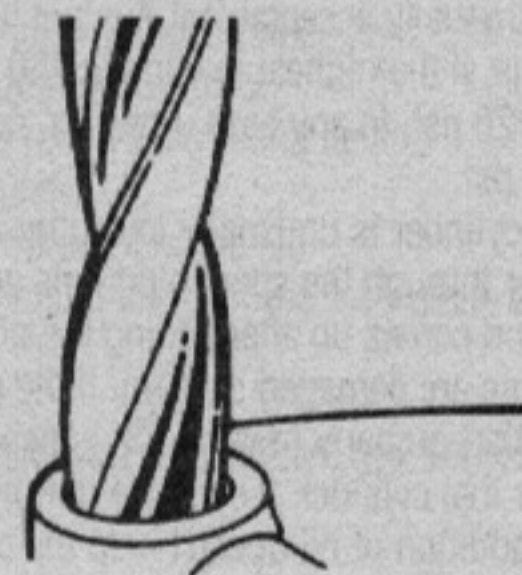
Fig. 36 Drill out the damaged threads with specified drill. Drill completely through the hole or to the bottom of a blind hole
