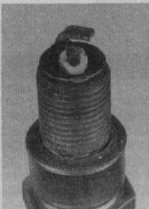
Fig. 8 Inspect the spark plug to determine engine running conditions
