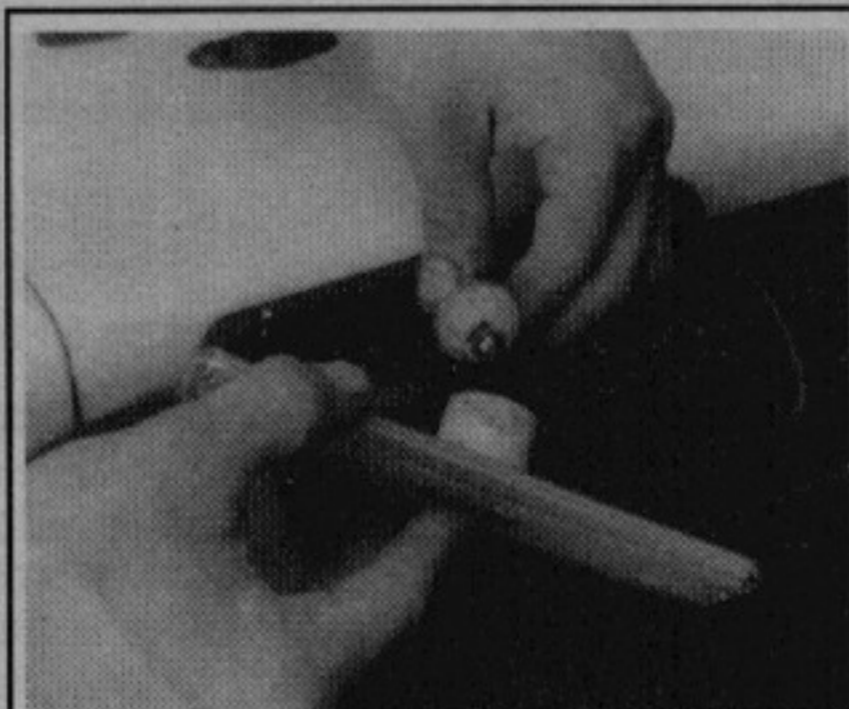
Fig. 75 Disconnect the bulb socket from the rear of the lamp
