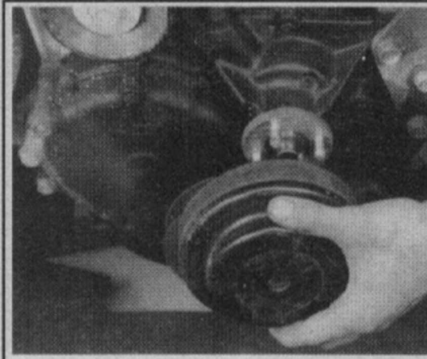
Fig. 88 Removing the fan pulley from the water pump
