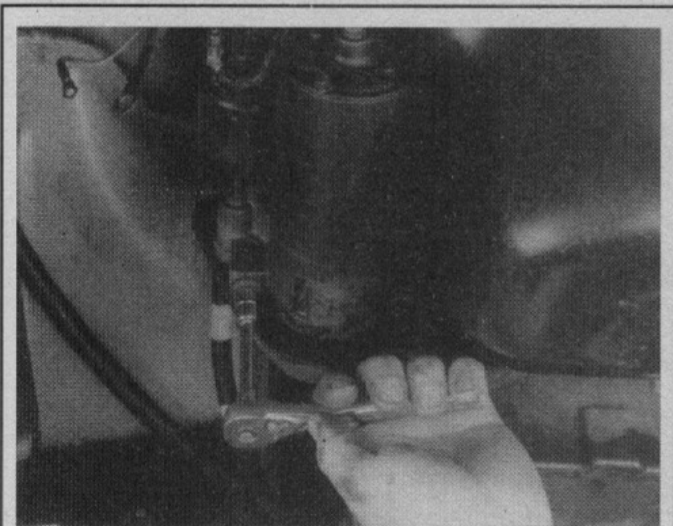
Fig. 32 Removing the starter outside mounting bolt
